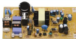
Discrete power supply: 70 components
