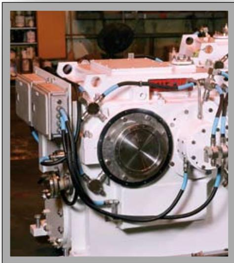
**Power Transmission Products and Services** LUFKIN IS ALSO A LEADING WORLDWIDE PROVIDER of power transmission equipment, primarily precision-made gears in weights of from 300 pounds to 250 tons and in power levels from 20 to 85,000 horsepower. These highly engineered products are used in industrial applications in a variety of industries, such as oil and gas,
