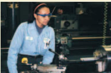
A machinist in the Memphis office makes a lineshaft for a vertical turbine pump that will be installed at a water well site.
