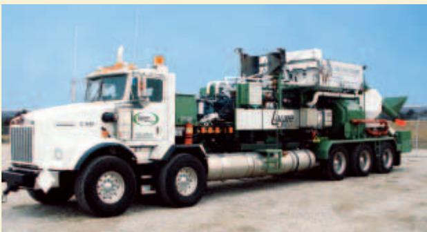
A 1,300 HP Custom Well Stimulation unit custom-built by Layne Energy is being used in the Midwestern United States for proprietary stimulation of coalbed methane wells.
