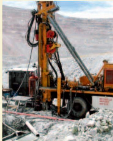
Fulfilling a three-year contract in northern Chile includes using a JKS Boyles B-20 diamond rig to drill at the mining site.
