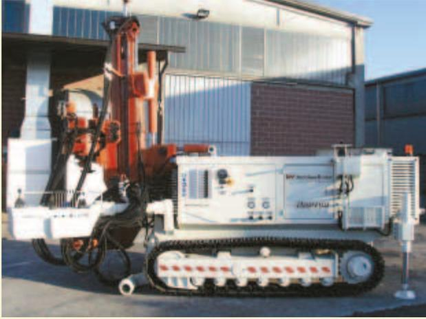
The track-mounted Techniwell TW1400 Raptor drill is designed for soil-improvement applications such as minipiles and can be used in low-headroom areas.
