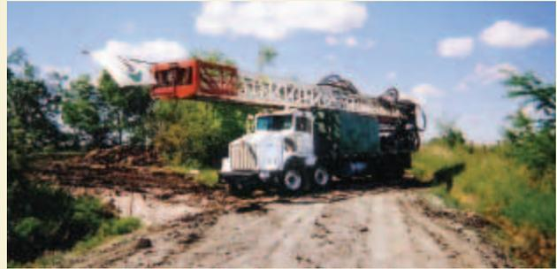
ATH150 Top Drive drill rig is used for large-diameter wireline coring and air drilling of coalbed methane wells up to 2,500 feet deep.
