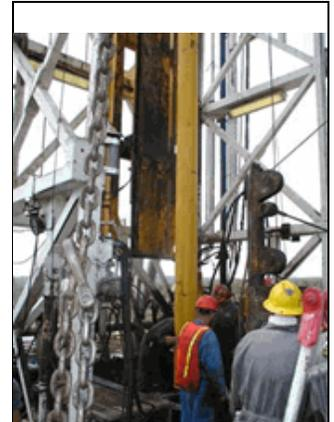
Rig crew running recess shoe for Baker Oil Tools' linEXX expandable liner system.
