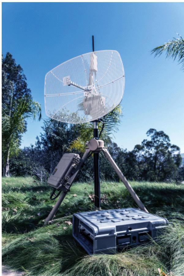
AeroVironment's new long-range tracking antenna for its Puma™ AE small drone lets warfighters gather surveillance data farther from dangerous hostile fire. (Photo: Business Wire)
