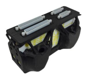
The weight of this Stratasys 3D printed circuit box for space applications was reduced by 30% using SIMULIA design optimization (Photo: Business Wire)
