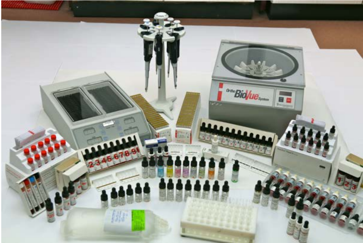
The Blood Bankers current “toolbox” – multiple reagents (gel cards, antibodies and red blood cells), significant consumable requirements - COMPLEXITY
