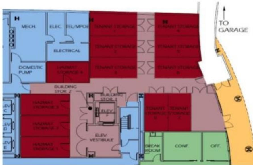
ONE TOWER PLACE – SECOND LEVEL HAZMAT STORAGE AREA PLAN
