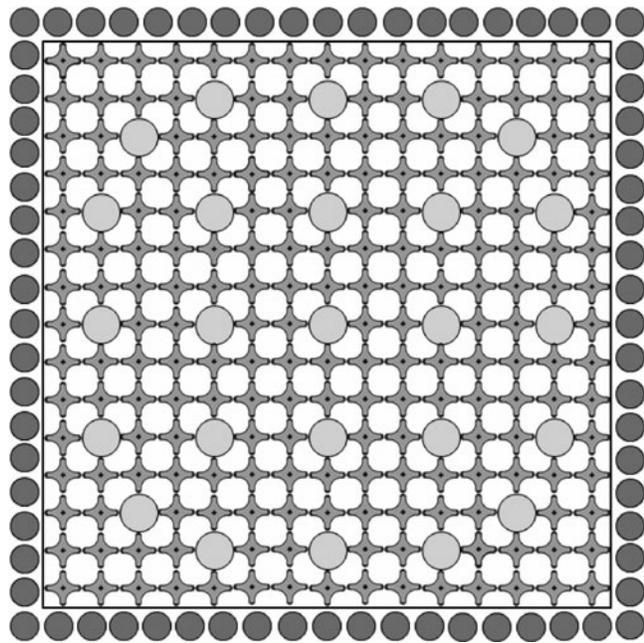
Fig. 3. Lightbridge's all-uranium seed-and-blanket fuel assembly for power uprate in existing  $17 \times 17$  PWRs. Central region contains helical-cruciform metallic fuel rods and control rod guide tubes. Peripheral row comprises pelletized  $\text{UO}_2$  fuel rods.
