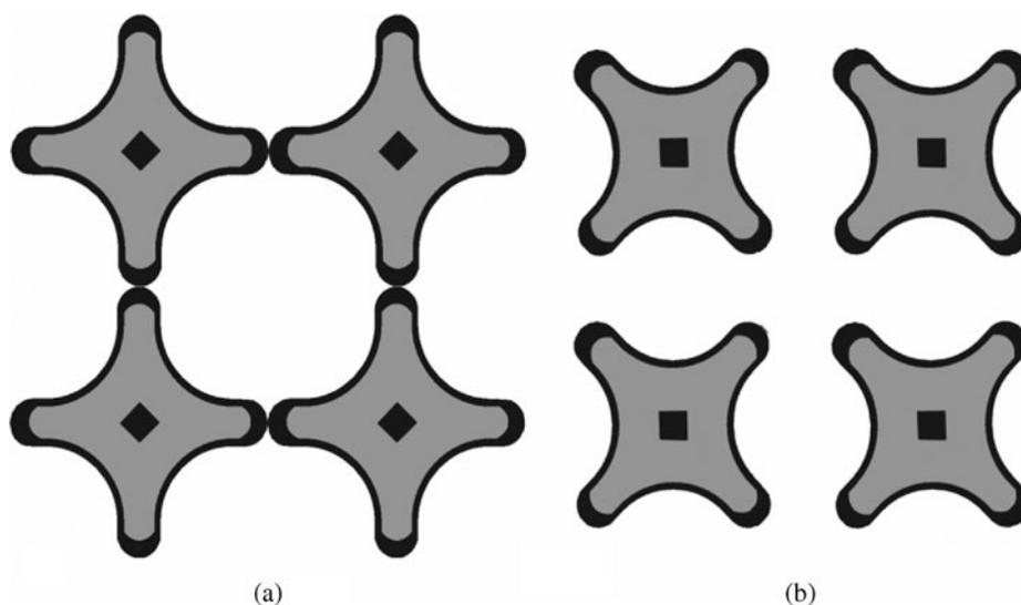
Fig. 2. Schematic cross section of the metallic fuel rod aligned in a square lattice array (a) showing the self-spacing plane wherein rod-to-rod contact eliminates the need for spacer grids and (b) axially halfway between self-spacing planes.
