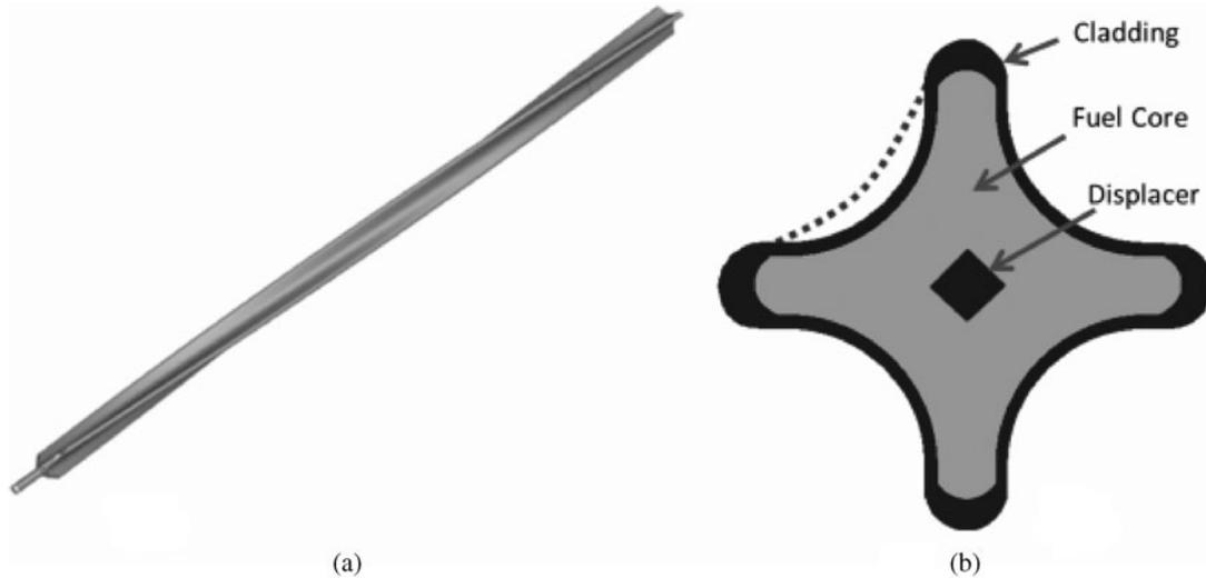
Fig. 1. Schematic of Lightbridge's metallic fuel rod for PWRs: (a) segment of rod showing helical twist and (b) cross section showing the fuel core, central displacer, and cladding. The dashed line identifies the typical change in fuel rod profile at end of life due to swelling deformation. (Not to scale.)
