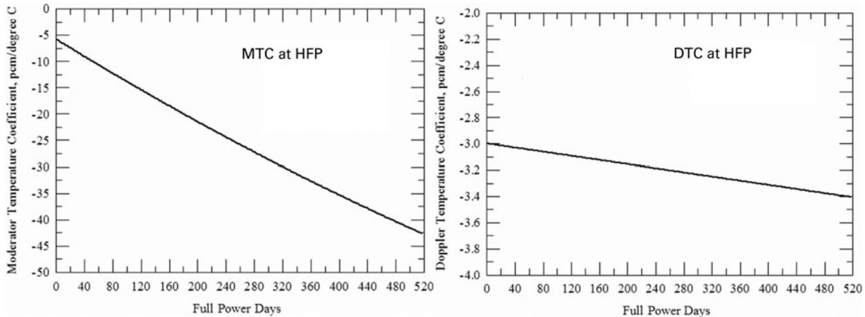
Fig. 4. MTC and DTC of reactivity for a typical PWR utilizing Lightbridge's all-uranium seed-and-blanket fuel assembly.
