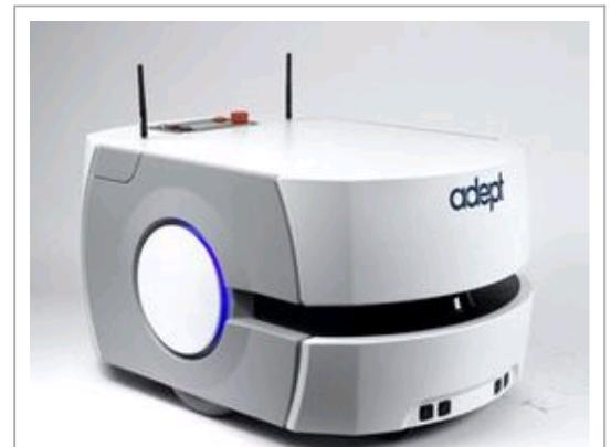
The Adept Lynx self-navigating Autonomous Indoor Vehicle (AIV) will be shown in Adept's booth 354 at Automate 2013, January 21 - 24 in Chicago IL. The AIV is designed for autonomously moving materials from point to point which may include confined passageways as well as dynamic and peopled locations.
