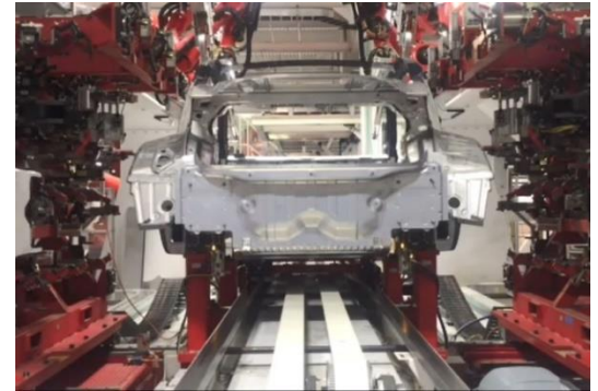
Model 3 Body Shop Welding (Video Embedded)
