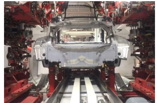
Model 3 Body Shop Welding (Video Embedded)
